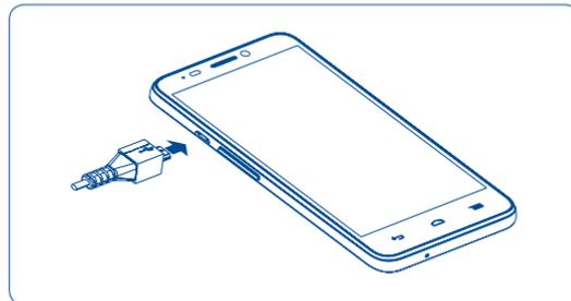
Connect the battery charger to your phone and mains socket respectively, LED indicator will light while charging.
