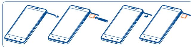
Insert the microSD card with golden contact facing downwards into the slot. To remove the microSD card, gently press and slide it out.
