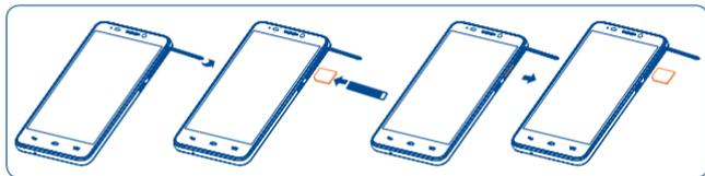
To install, place the SIM card chip facing downwards, and then slide it into its slot. Make sure that it is correctly inserted. To remove the card, press and slide it out.
