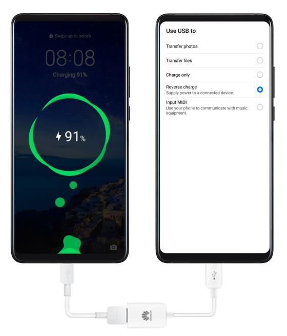
You can use your device to charge other devices using an OTG cable.
