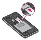
3 Insert the battery into place by aligning the gold contacts on the phone and the battery (1) and pressing it down until it clicks into place (2).
