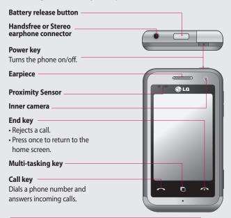
MARNING: Putting a heavy object on the phone or sitting on it can damage its LCD and touch screen functionality. Do not cover the protection film on proximity sensor of LCD. It can be caused the malfunction of sensor.
