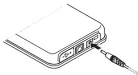
The charging time depends on the charger used. Charging a BL-4C battery with the AC-3 charger takes approximately 2 hours and 45 minutes while the device is in the standby mode.
