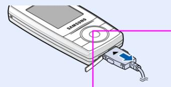
**Note:** Do not remove the battery from the phone without unplugging the adapter first. Otherwise, the phone may be damaged.
