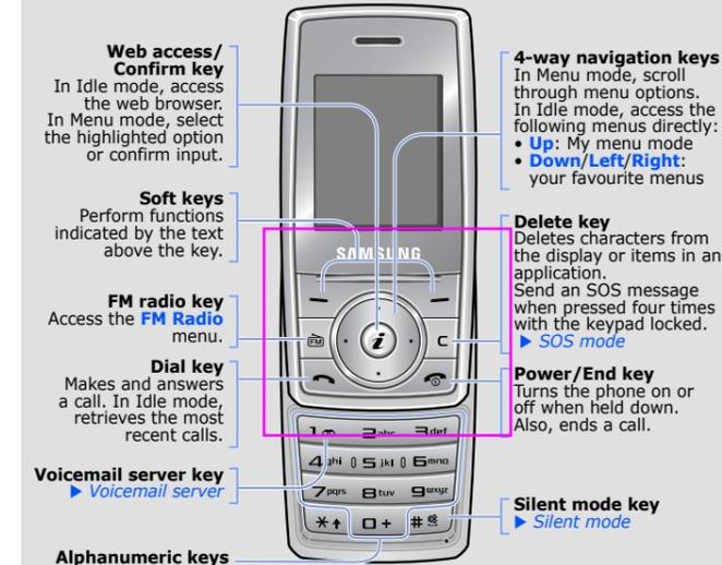
**Silent mode** Press and hold **\*** in Idle mode to disable all sounds on the phone. To exit, press and hold this key again.
