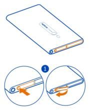
2 To unlock the card holder, slide the holder to the left. Carefully pull out the holder.
