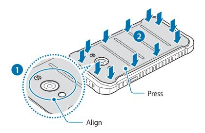
Ensure that the back cover is closed tightly to prevent water and dust from entering the device. Open or loose back cover may allow water and dust to enter the device and cause damage.
