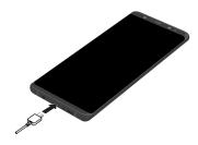
**Caution**: Use only charging devices and batteries approved by Samsung. Samsung accessories are designed for your device to maximize battery life. Using other accessories may void your warranty and may cause damage.
