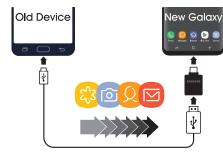
**Note**: The USB option must be set to Media device (MTP) on the other device. Transferring content with a USB cable may increase battery consumption. Make sure your battery is fully charged.
