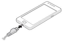
Connecting the travel adapter improperly may cause serious damage to the device. Any damage caused by misuse is not covered by the warranty.
