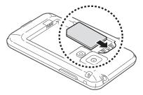
The antenna is located in the upper area on the back of the device. Do not remove the protective tape covering the antenna, as this can damage the antenna.
