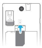
• Remove the battery cover, then insert the SIM card into its slot with the goldcoloured contacts facing down.
