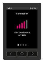
Like your phone, the gateway displays up to five bars on its Connection screen, indicating signal strength.
