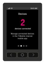
The Devices screen indicates how many devices are currently connected to the gateway. This is true for both wireless and wired devices.
